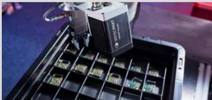
The VISOR® Robotic detects the position of the component in a load carrier and transmits the gripping position directly to the robot.
