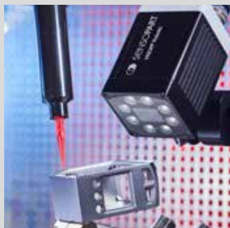
The VISOR® Robotic determines the exact position of the sensor housing. Offset data is used to correct the robot's trajectory.
