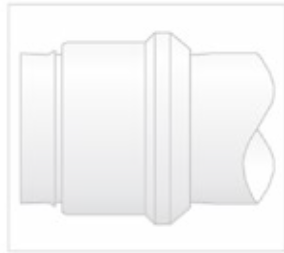
Fig. T48 — Shallow bite
