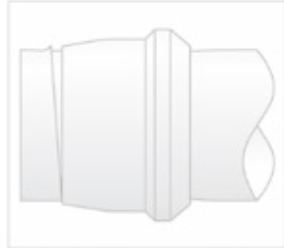
Fig. T50 — Ferrule cocked on tube
