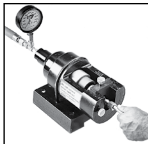
Fig. S27 – Flaring with Hydra-Tool
