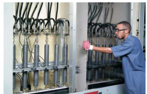
Every accumulator is cycle tested prior to shipment.
