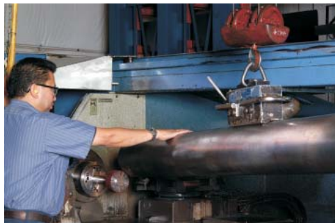
Large bore piston accumulators are machined on large capacity lathes.
