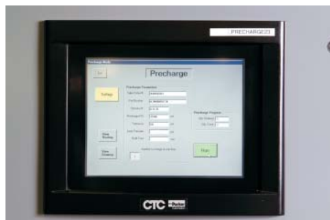
Parker's in-house designed pre-charge machine ensures proper pre-charge regardless of ambient temperature.
