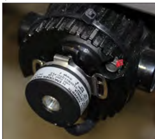
BELOW: A Model 15T mounted on the end of a motor. See page 40 for product specifications.
