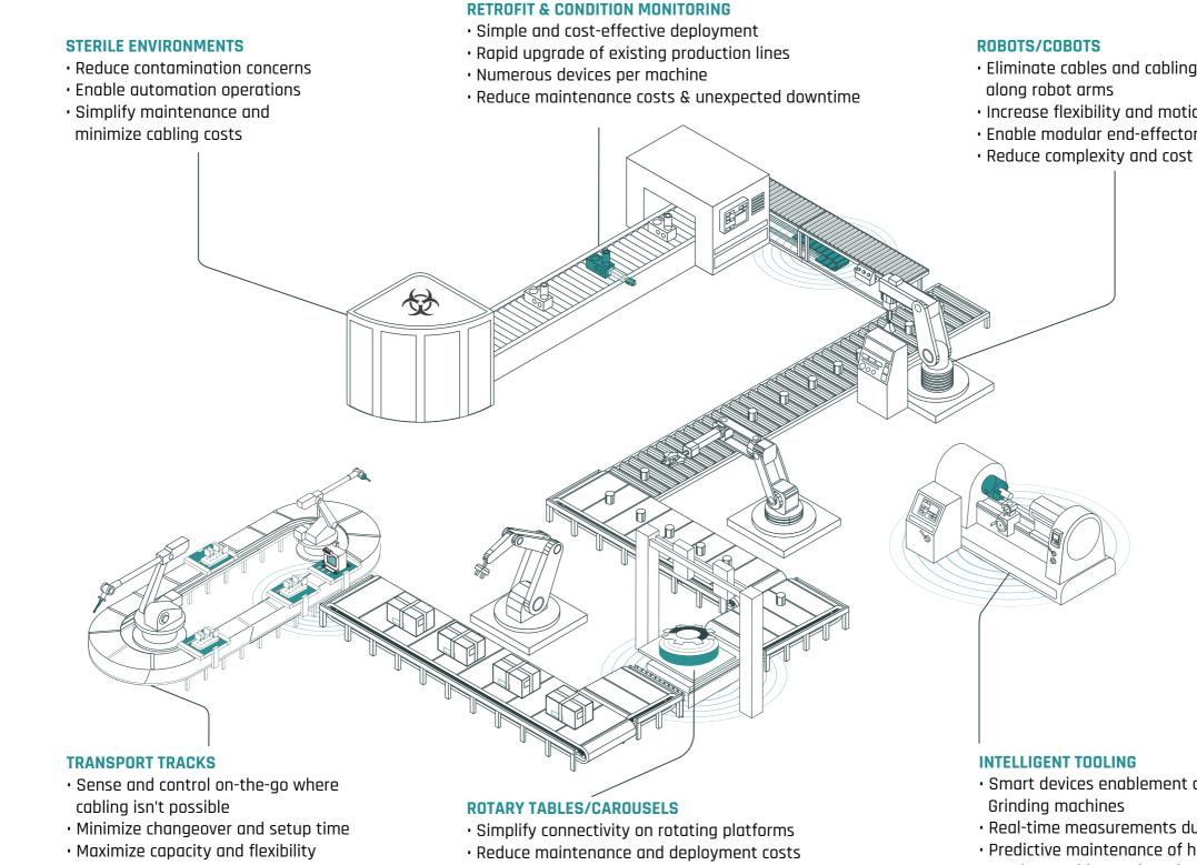
Flexible configuration and setup
