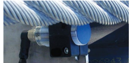
Distance monitoring for position control
