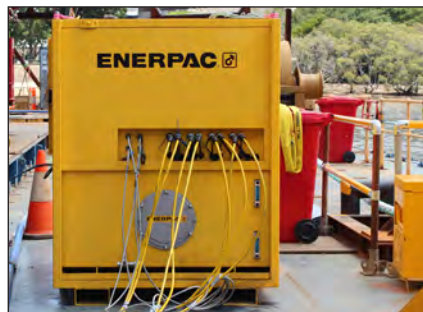
▼ SyncHoist Powerpack to operate the 4 lifting points.
