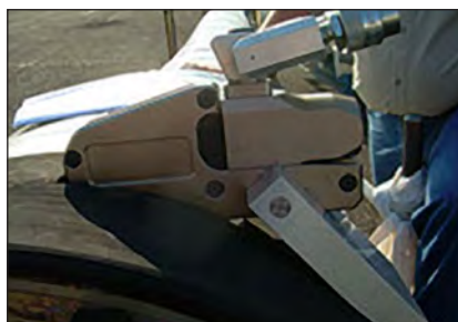
◀ Custom hydraulic torque wrenches with reaction paddles for use with a flexible flowline.
